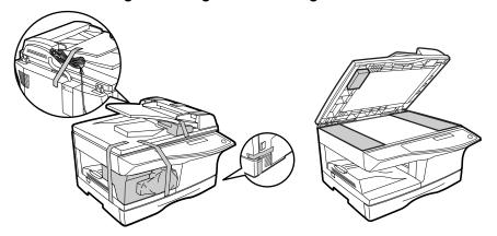
3 Release the scan head locking switch.
